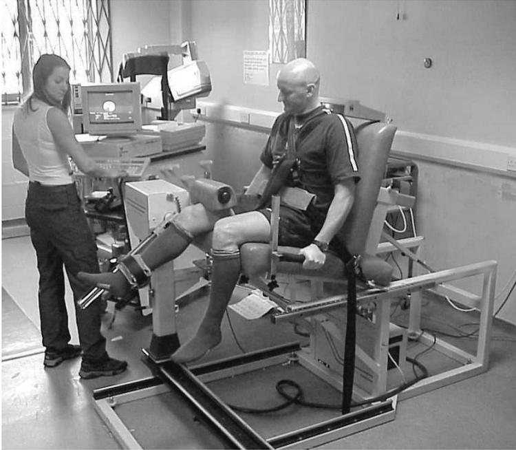
*Figure 3.1* Isokinetic dynamometer (Lido) for measurement of muscular function in isometric, concentric or eccentric modes.
