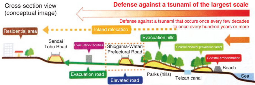
Fig. 5.15 Cross-section view of coastal area reconstruction and basic concept for preventing tsunami damage for the city of Sendai (Sendai City 2016)
