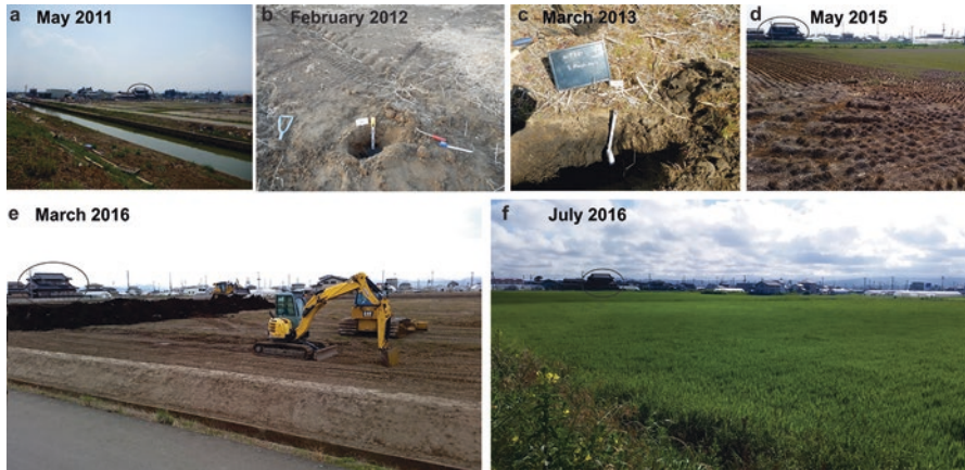
Fig. 14.6 Site B – May 2011, February 2012, March 2013, May 2015, March 2016, July 2016. See Fig. 14.1b for site location. The black ellipse marks the location of the house in photos taken in May 2011, May 2015, March and July 2016. In March 2016, the soil above the hard pan was removed and new organic-rich soil laid down (Photos Catherine Chagué-Goff)
