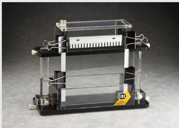
FIGURE 1. Typical apparatus used for vertical polyacrylamide gel electrophoresis. The gel is cast between the two glass plates, which are separated by thin plastic spacers and held together by the paper clips. The “comb” at the top will be removed, leaving wells into which the samples will be loaded.
