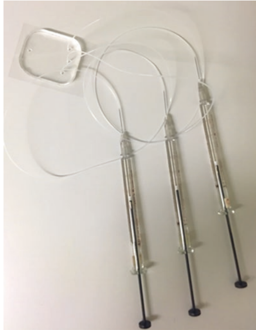
Fig. 3 The ready-to-use microfluidic device. The transparent microfluidic device covalently bonded to a coverslip and connected to three glass syringes through plastic tubing
