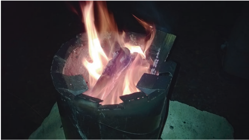
Fig. 9.1 A simple and robust cooking stove. Note: The stove quickly produces a hot flame using a small amount of wood. The idea is simple: cooking with an efficient stove spares fuelwood and saves forests. Source: Photo by the author
