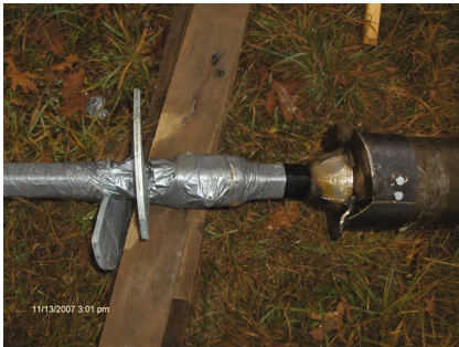
Fig. 5. FRP-G-HSP Pile prior installation
