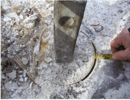
Fig. 15. FRP-G-HSP (external grout) After cyclic lateral testing
