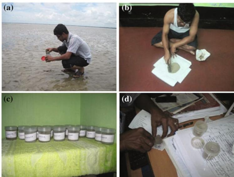
Fig. 4.2 Sediment sample collection (a), preparation of sediment samples (b), prepared sediment samples (c) and sample pressed in sample holder (d)
