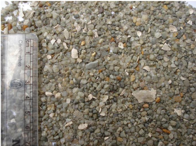
**Fig. 4.15** Sand sample of aquifer A5 at Paradeep (225 mbgl)
