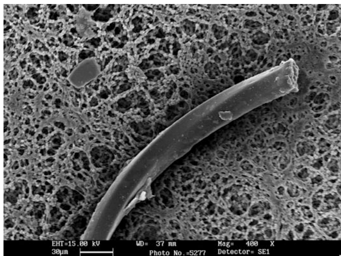
Fig. 5 Microplastic (on PVDF filter) obtained from filtration of washing effluents
