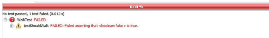
Figure 13-2. Netbeans IDE displaying a unit test failure
