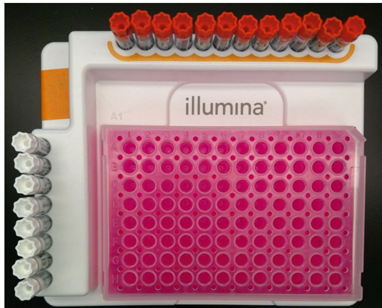
Fig. 8 Nextera ® XT dual indexing set up. Nextera ® XT index set up using Illumina's TruSeq Index Plate Fixture. Index 1 (i7) goes across the top of the plate ( orange caps ) while Index 2 (i5) goes vertically down the side ( white caps ). Add i7 indexes down each column and add i5 indexes across each row. If making less than 12 libraries please see the Illumina low plexing guidelines
