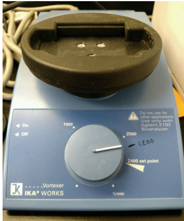
Fig. 6 Modified IKA vortexer settings. The IKA vortexer should be set to ~2200 rpm when vortexing a DNA chip to avoid marker carryover from one well to the next. Estimate the middle of the two set points (2000 and 2400) on the vortexer, draw a line and manually set your knob to that speed
