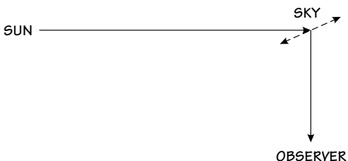
FIGURE 4.20 The light radiated by a patch of sky is polarized in the direction of the dashed line, that is, at right angles to the direction of the Sun.
