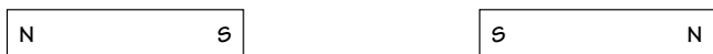
FIGURE 3.3 Two nearby magnets. The sum of the repulsions between the north poles and between the south poles is greater than the sum of the attractions between the unlike poles.
