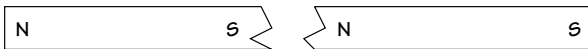
FIGURE 3.5 Cutting a magnet in half. Two new poles appear, so that two half-length magnets result.
