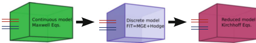
Fig. 5.12 Three levels of abstraction for a component model and its corresponding equations
