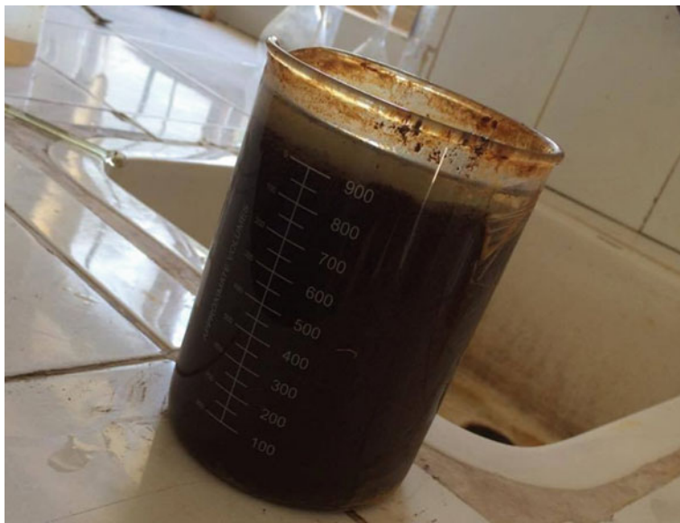
Fig. 10.1 Coagulated sludge from industrial wastewater
