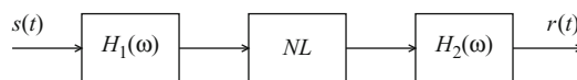
Fig. 4.6 The BPNL structure: a time-invariant nonlinearity NL is placed between two bandpass filters, H_1(\omega) and H_2(\omega) . The first limits the input frequency band, the second reduced harmonic distortion (overtones), but allows intermodulation within the passband
