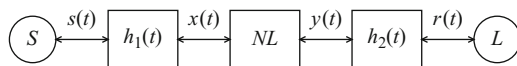
Fig. 5.1 The time domain version of a simple BPNL structure: a nonlinear element NL is placed between two linear elements with impulse responses, h_1(t) and h_2(t) . The first has the properties of a band-pass filter, the second is a simple low-pass element which reduces distortion product harmonics (overtones). Stimulus source properties and load properties also play a role (Elaborated in the text)
