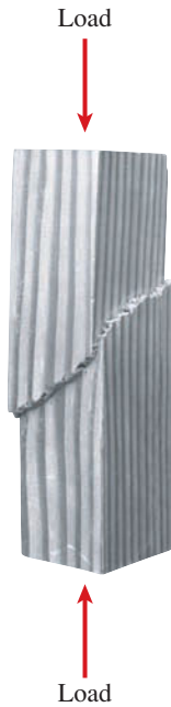
FIG. 2-37 Shear failure along a 45^\circ plane of a wood block loaded in compression
