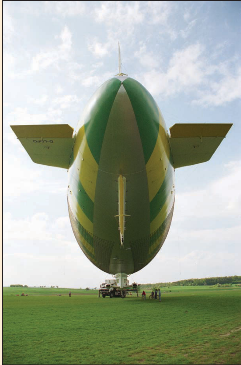
Airships such as this blimp rely on internal pressure to maintain their shape using a gas lighter than air for buoyant lift.
