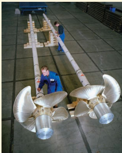
Ship drive shaft is a key part of the propulsion system
