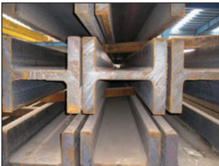
The centroid of wide-flange steel sections lies at the intersection of the axes of symmetry
