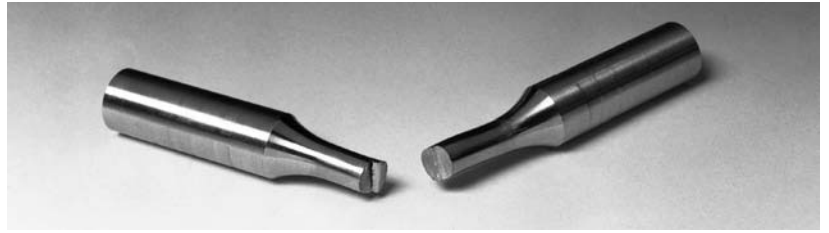
FIG. 2-57 Fatigue failure of a bar loaded repeatedly in tension; the crack spread gradually over the cross section until fracture occurred suddenly. (Courtesy of MTS Systems Corporation)
