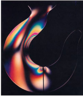
(b) Photoelastic fringe pattern
