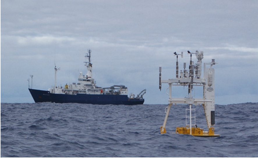
Fig. 10 The Research Vessel Melville sitting next to a surface buoy deployed under the marine stratus clouds 800 nm west of northern Chile. The ship is holding bow into the wind near the buoy to support intercomparison of shipboard meteorological data with that from the buoy. Note the bow tower mounted on RV Melville just aft of the jackstaff to provide a place to mount the ship's sensors
