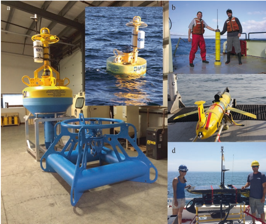
Fig. 2 Some near real-time passive acoustic monitoring platforms, including (a) moored buoy, (b) profiling float, (c) Slocum ocean glider, and (d) wave glider. Photographs (a, b, d) copyright Woods Hole Oceanographic Institution, (c) copyright The Nature Conservancy
