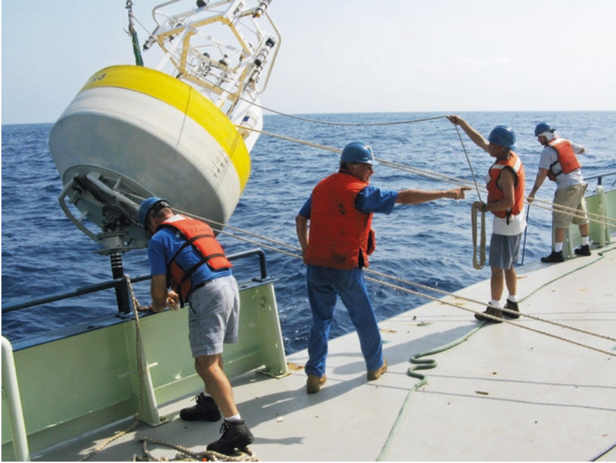
Fig. 4 Photograph showing the underside of a surface buoy to illustrate the mechanical/electrical connection between the subsurface components and the surface buoy. A special universal joint can be seen just under the buoy. The component bolted to the underside of the universal joint ( black hose ) is the potted EM chain assembly consisting of high-strength chain with a spiral wrapped cable all potted in a marine exhaust hose (Photo credit: Alex Dorsk, Woods Hole Oceanographic Institution)
