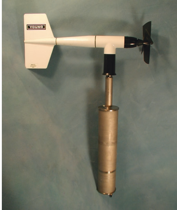
Fig. 1 R.M. Young Marine Wind Monitor Model 05106 fitted to an ASIMET module. Titanium tubing used for the housing has an outside diameter of 3.5 inches (8.89 cm)
