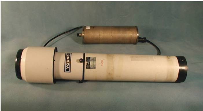
Fig. 7 An RM Young Model 50,202 self-siphoning rain gauge attached to an ASIMET module that digitizes the 0–5 volt DC output of the rain gauge can record data and can provide communication capability
