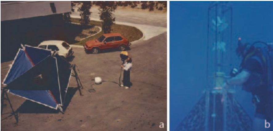
Fig. 2 (a) SVP drifter with TRISTAR drogue with Dr. Peter Niiler holding the surface buoy. (b) Diver checking the current meters used to measure the slip of the TRISTAR drogue through the surrounding water
