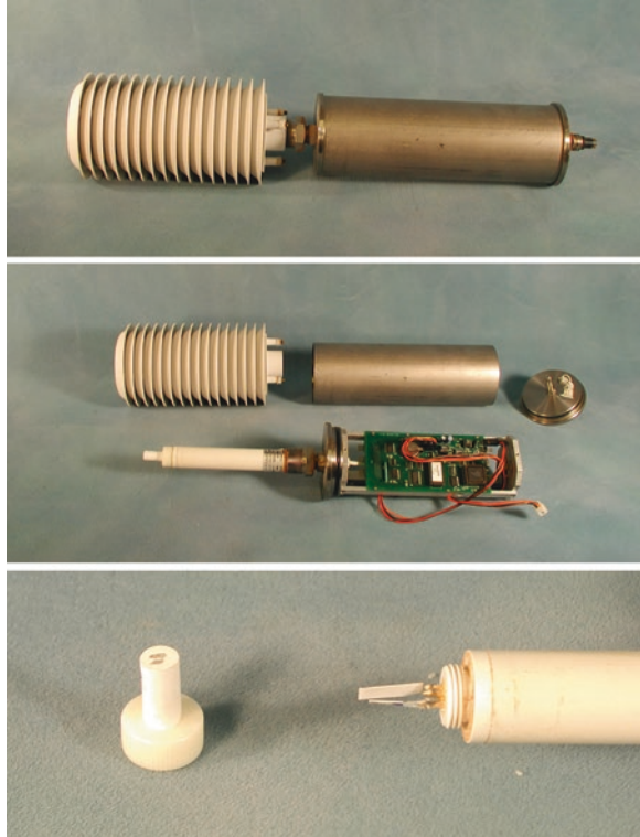
Fig. 3 Two pictures of the relative humidity/air temperature sensor module and a close-up of the sensor assembly. Top: assembled, with Gill multiplate radiation shield over sensor assembly; Middle: sensor module removed from tube and radiation shield; Bottom: Close-up of the sensor assembly showing the white, capacitive thin film humidity sensor, and, difficult to see, a thermistor temperature sensor
