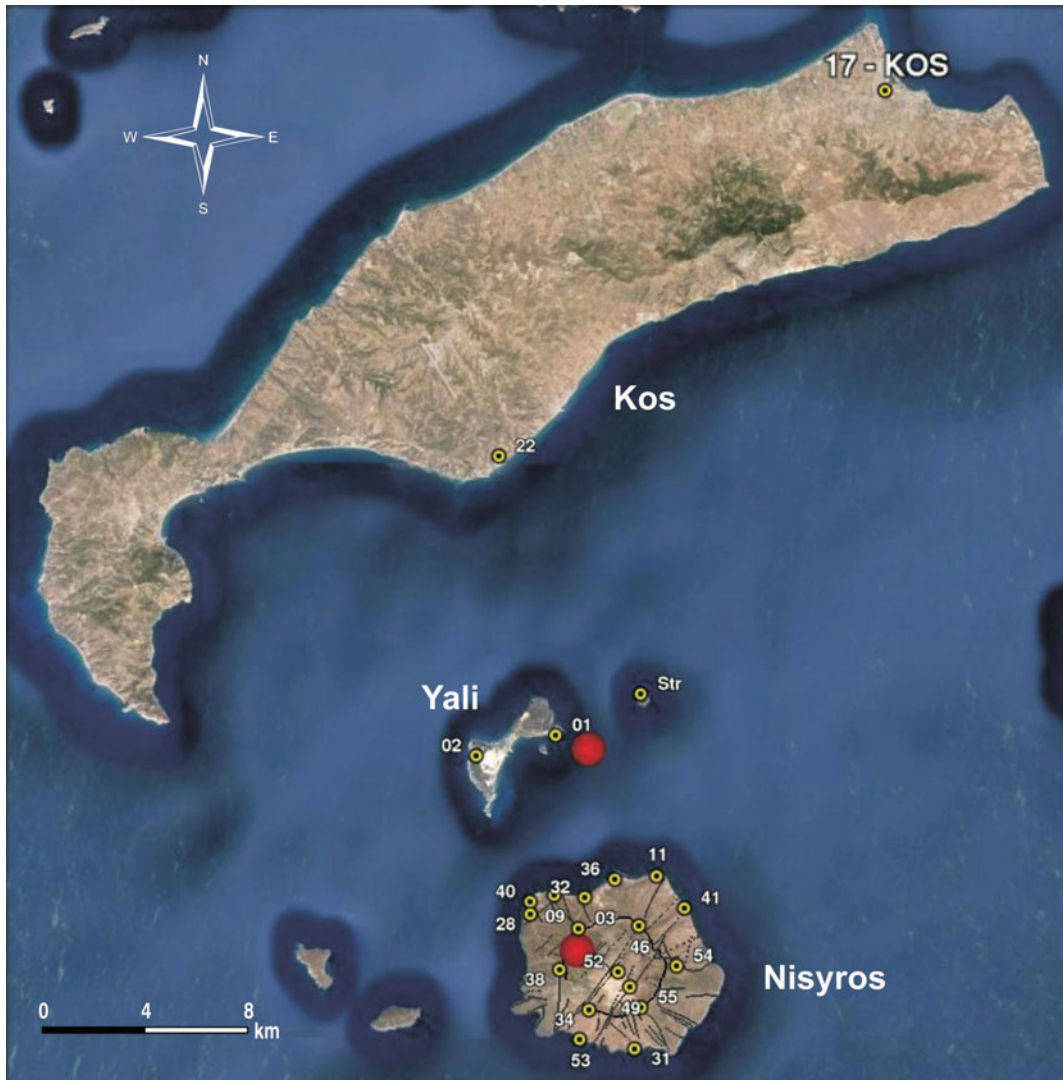
Fig. 10.1 Distribution of stations of the GPS network of the Kos-Yali-Nisyros Volcanic Field. Solid red circles represent the two modelled Mogi point sources. Str stands for the station established on Strongyli Islet
