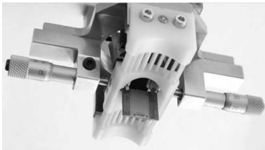
Fig. 11: POM-made tilt-module with gripper unit
