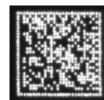
Fig. 7. Dots of 4 times high density compared with Fig.3 (b). Dot pitch: 60 \mu m. Size: 1.66 mm.
