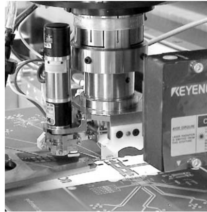
Fig. 12: Tilt-gripper with HarmonicDrive® mini-servo in assembling position
