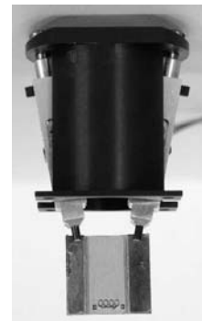
Fig. 9: The gripper unit with the two micro-finger grippers
