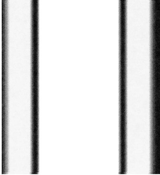
Fig. 7 The single-slit diffraction pattern.
