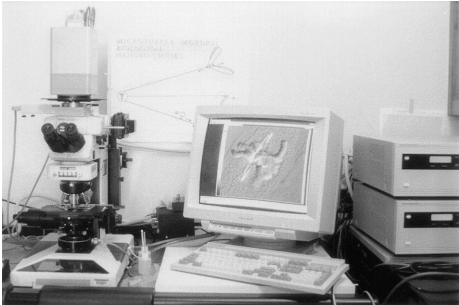
Fig. 1 Photograph of the multimode digital imaging system including the Nikon FXA upright microscope sitting on an air table (Newport Corp., Irvine, CA, VW-3660 with 4-inch-high tabletop). Images are captured with a Hamamatsu C4880 cooled CCD camera. Image acquisition, storage, processing, analysis, and display are controlled by MetaMorph Digital Imaging software in a Pentium-based computer.
