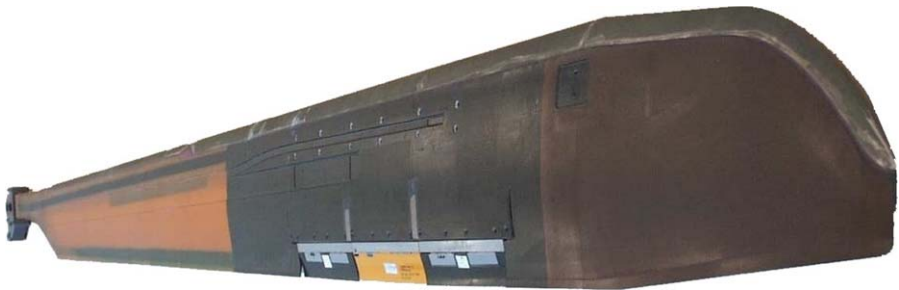
Fig. 2.8. Experimental rotor blade with trailing edge flaps; from Klöppel et al. [112].
