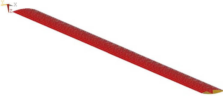
Fig. 10.11. Discretization of the convex cross-section beam with shell finite elements.
