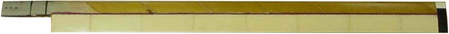
Fig. 2.9. Scaled active twist rotor blade with piezoelectric fiber composite patches attached to the spar; from Cesnik [44].
