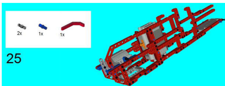
Figure 7-27. A Connector Peg is placed on one of the 4 x 2 Angular Beam on the right side of the construction, and the Double Angular Beam joins with a vertical 5M Beam on the same side.
