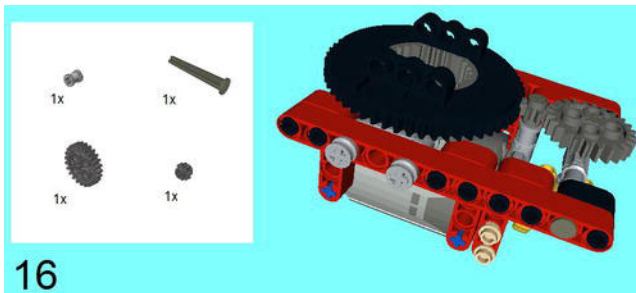
Figure 6-17. Another 4M with Stop and Bush join with the 180 Degree Angle Element in front of the construction. Now that this is secured in place, put the Gears on it as shown, and be sure they mesh together.
