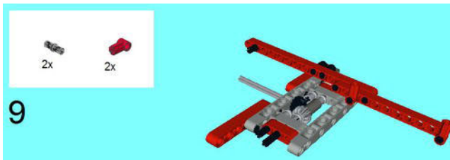
Figure 5-59. This Zero Degree Angle Element and two Connector Pins will come into play later in Step 47 to hold the engine for propulsion.
