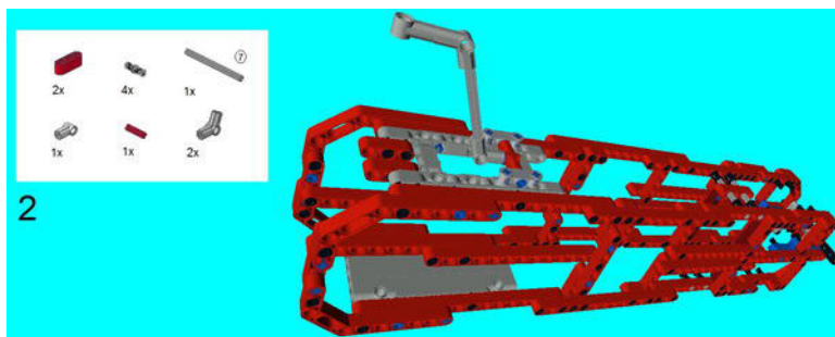
Figure 7-95. Add on two 112.5 Degree Elements with the 7M Axle, and the Zero Degree Element as well. Attach the 3M Beams with the four Connector Pegs.
