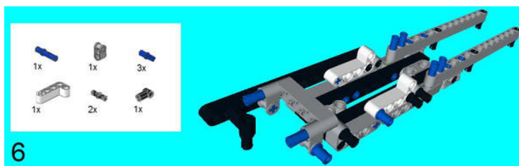
Figure 7-72. Attach a Cross Block to the 5M Beam as shown, and a Zero Degree Element to the 13M Beam. Don't forget to place the 4 x 2 with Connector Peg and Connector Peg/Cross Axle as shown.
