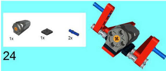
Figure 5-47. Add a 2 x 2 Plate on the 2 x 6 Plate and place the M-Motor over the entire 2 x 6 area. The 3M Connector Pegs go on the side as shown.
