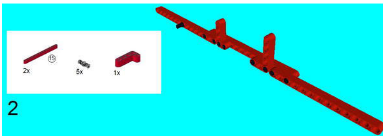
Figure 7-4. Join together two 15M Beams with the Connector Pegs and the 4 x 2 Angular Beam.
