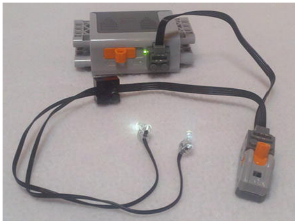
Figure 4-5. This is probably the most useful and simplest way of hooking up your lights with the Power Functions Control Switch.
