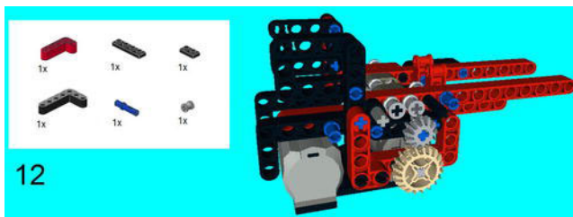
Figure 6-71. Apply the 1 x 4 and 1 x 2 Plates on the bottom of the M-Motor on this side to fill in the gaps below. Connect the 5 x 3 Beam to the 13M Beam with the 3M Connector, and attach the 4 x 2 Beam as shown. Don't forget to apply the Bush.
