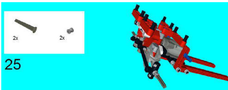
Figure 5-48. The section with the motor attaches to the steering section. The 4M Axles with stop also attach to the Steering Arms, along with the Bushes.
