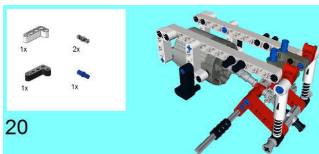
Figure 5-21. This Step is exactly like Step 19, but on the other side of the construction.
