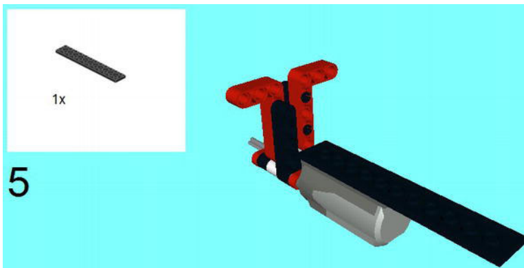
Figure 3-35. A 2 x 12 Flat Plate is required to click on the motor in 12 places, covering half of the plate.
