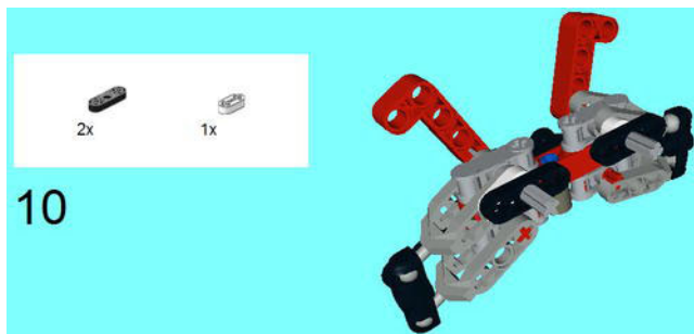
Figure 5-33. Add another 2M Lever on the other side, and two 3M Levers here.
