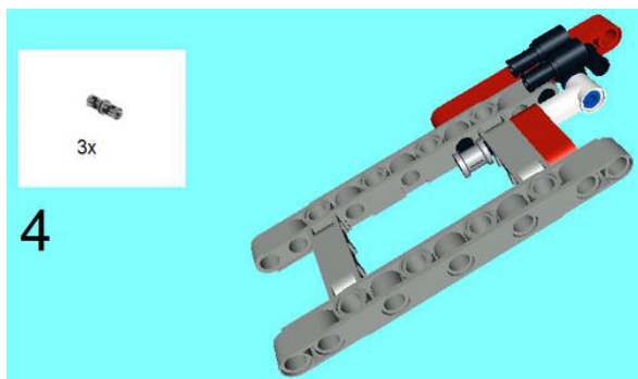
Figure 5-54. Two of the Connector Pegs go in the Technic Cross Axle and the third goes in the 7M Beam as shown.
