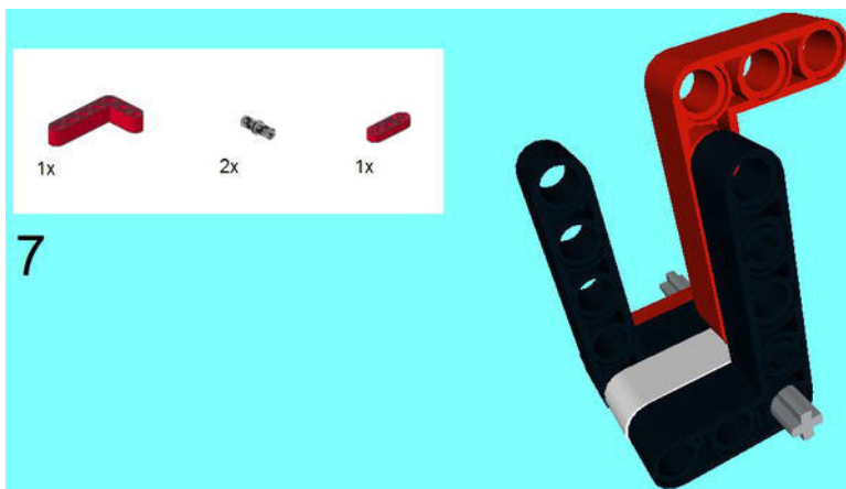
Figure 3-37. Attach a 5 x 3 Beam and 3M Lever. There should be a 1/2 M of Axle on one side and 1 M of Axle on the other.
