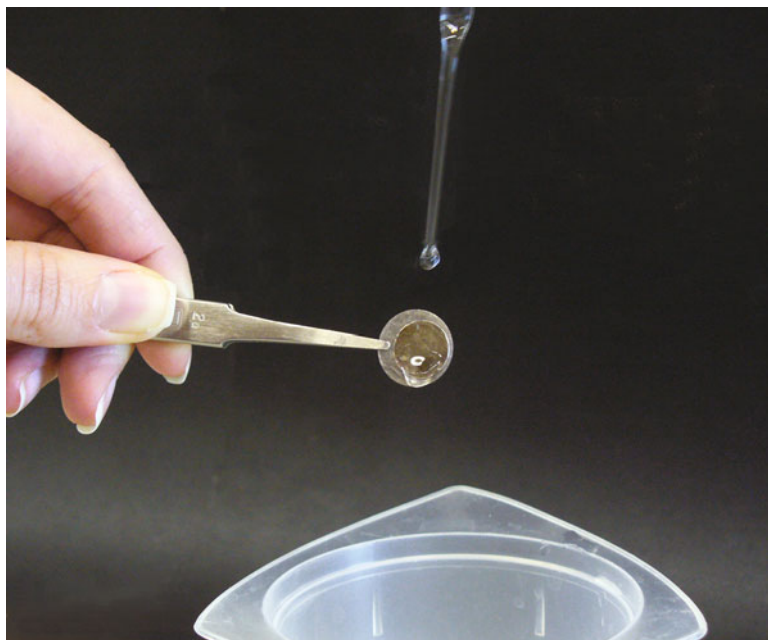
Fig. 2 Washing mica surfaces with water. The sample substrate is held by forceps on the edge of the metal disc, not over the mica. Water or buffer is washed over the surface using a pasture pipette
