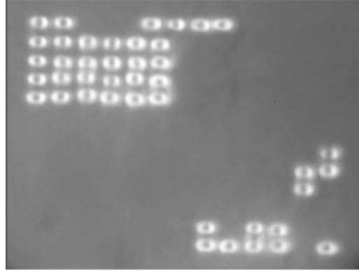
Fig. 6 Microscopy image of the time-shared optical trapping of 42 beads using AODs. This image demonstrates the smallest game of Tetris ever played. The corresponding video can be found online at https://www.youtube.com/watch?v=jCdnBmQZ6_s
