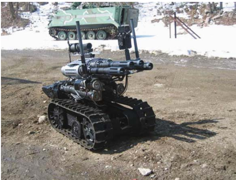
Fig. 4.5 Metal storm, a potential MPM-NLWS, mounted on the TALON mobile unmanned ground vehicle (UGV)
