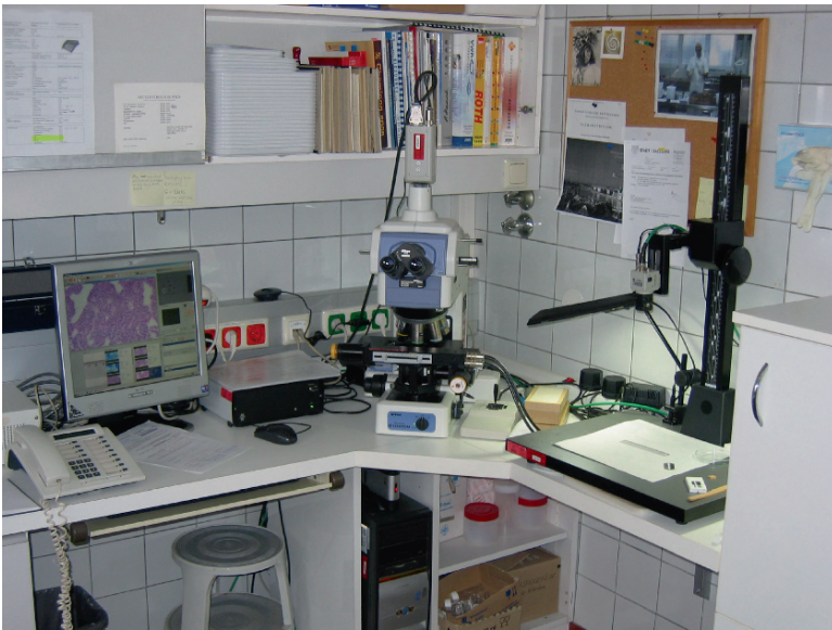
Fig. 4.9. Actual setup of the neuropathology laboratory. The smear preparation is stained (methyl blue) and placed under the robotic microscope (Fig. 4.8). An overview image is done at 0.5 \times magnification and the diagnostic areas are identified. These are scanned with light microscopy, and ideally the diagnosis is established
