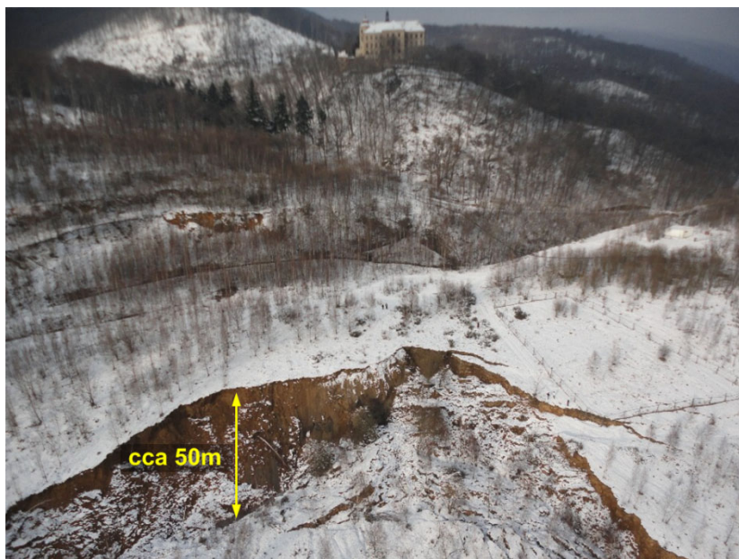
Fig. 7. Landslides at the pillar protecting the castle [11]
