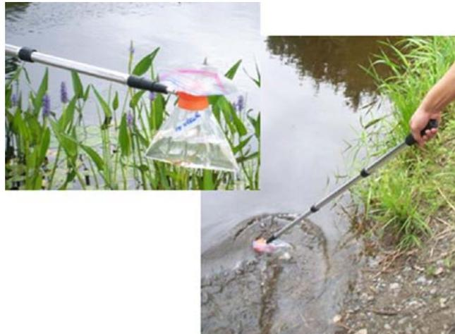
**Fig. 4** Collecting water samples in 1-quart bags using a telescoping golf-ball retriever. The retriever allows the collection of a bulk sample while also stirring the substrate. (For color version of this figure, the reader is referred to the web version of this book.)
