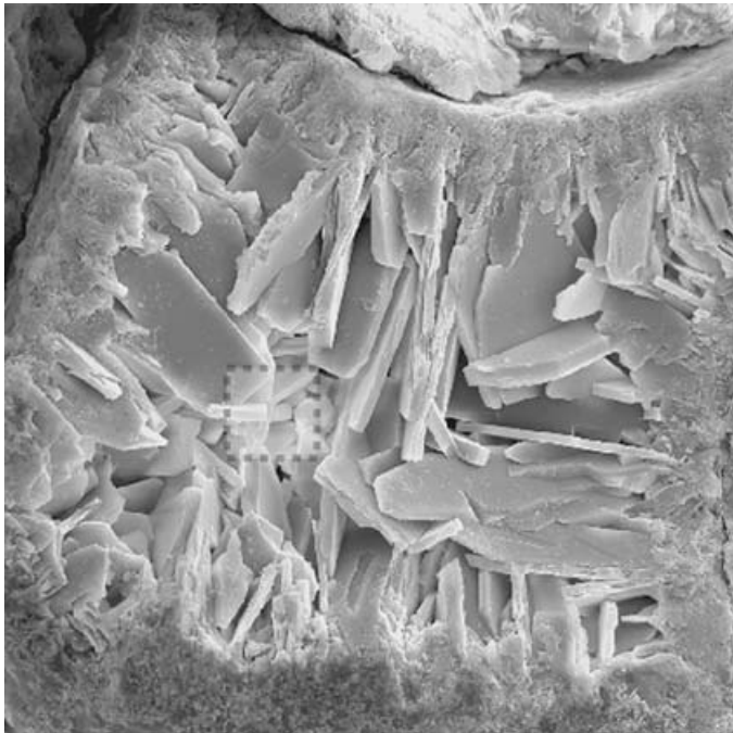
Plate 4.11. Stereoscopic image ( 400\times 400\ \mu\text{m} ) of clinoptilite crystals (view with red/green spectacles).
