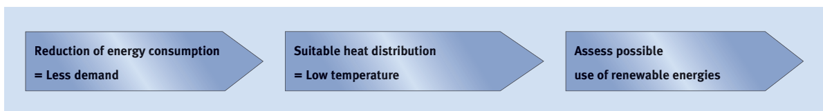
Fig. 3–74 Three steps towards an energy-efficient building
