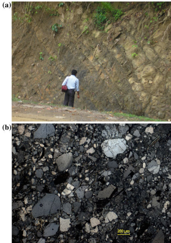
Fig. 7 Field and petrographic attributes of Andaman Flysch from Great Nicobar Island. a Section of Andaman Flysch exposed at road cutting near Campbell Bay observed by Anindya Bhattacharya (senior geologist). Note the parallel-sided, unchannelized and internally structureless medium thick beds of sandstone alternate with dark grey shale. b XPL microphoto of sandstones reveals textural immaturity and poor sorting of the framework grains loosely packed in argillaceous matrix
