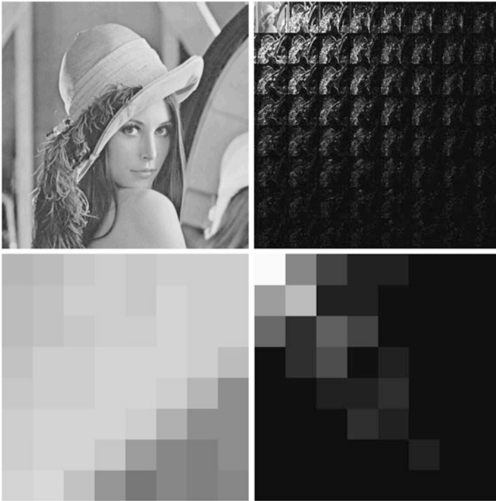
Fig. 12.12 Original image of Lenna and its bidimensional DCT. Below: an example of 8 \times 8 block of Lenna and its DCT (courtesy of Roberto Rinaldo)
