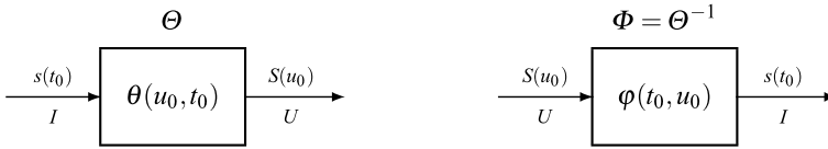
Fig. 14.4 Domains, functions, and kernels of the transform and its inverse
