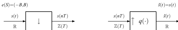
Fig. 8.15 Exact signal recovery from its samples by an interpolator filter under the hypothesis of band limitation and F_c \geq 2B
