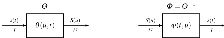
Fig. 14.1 Domains and kernels in a general transform and in its inverse transform
