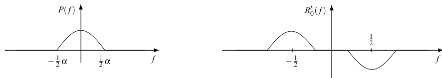
Fig. 9.27 Derivative R'_0(f) of raised cosine for \alpha = 0.6
