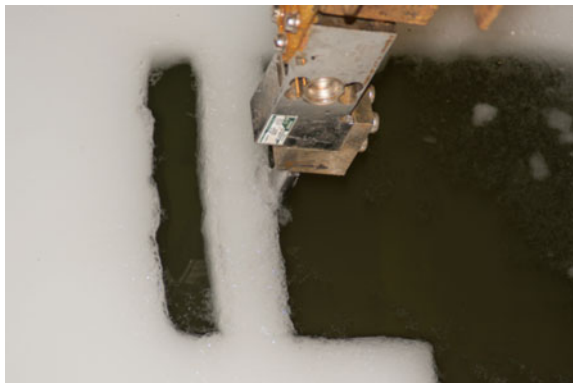
Fig. 3 The rig for tests on sea ice (in the air and submerged into the water before the tests)
