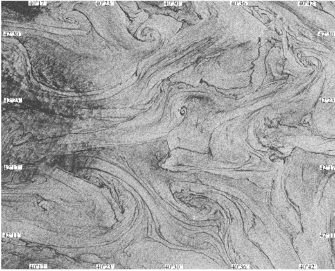
Fig. 9 Manifestation of submesoscale eddies in a radar image of the sea surface during autumn phytoplankton bloom in the eastern part of the Black Sea. A part of a Sentinel-1A image of October 26, 2014, 03:24 UTC
