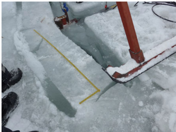
Fig. 10 Fracture pattern after the test. Beam #Sea2_L, \frac{L}{h} = 5.5 (Table 1)
