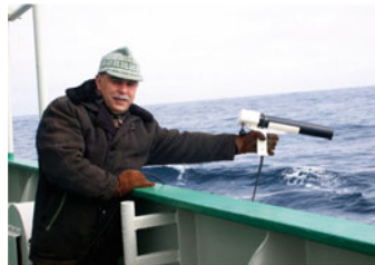
2002: Drake passage, shooting an XBT sensor
