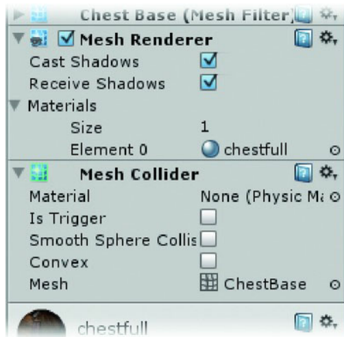
Figure 7-44. The generated Mesh Collider
