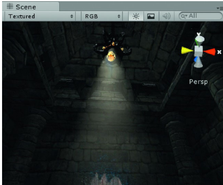
Figure 14-39. The fake volume light using the Line Renderer
