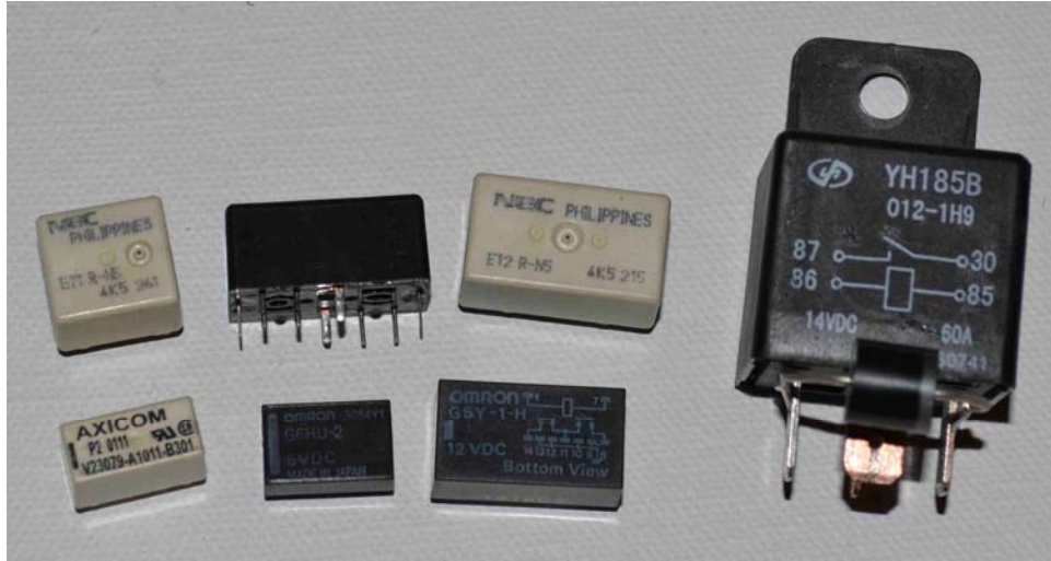
Figure 2-1. Here you can see a variety of relays in small to large sizes. The three smaller relays on the bottom row are called “signal” relays, meaning their contacts are rated for less than 2 amps of current. The three relays on the top row are called “power” relays, ranging from 5 amp to 25 amp contact ratings. Lastly, the mammoth relay on the far right is an automotive power relay, which is rated at 60 amps.
