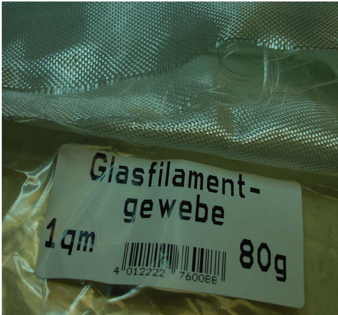
Figure 9-2. Woven fiberglass fabric with 80g/m 2
