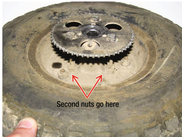
Figure 10-5. The rear wheel with sprocket installed
