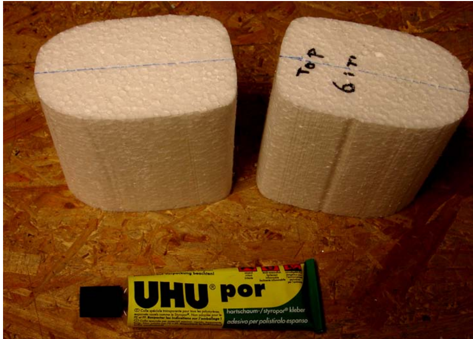
Figure 9-13. Two adjacent segments with EPS/XPS glue
