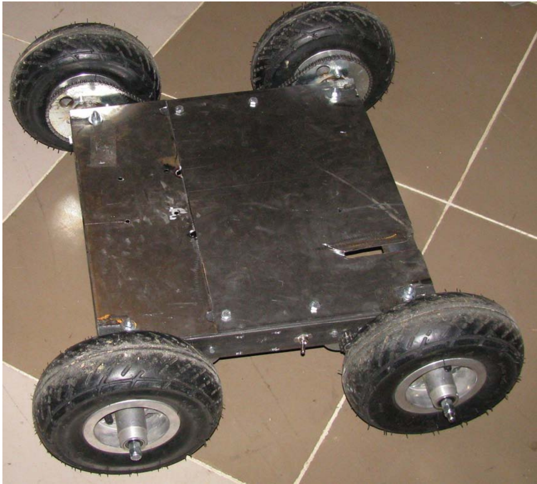
Figure 12-24. The basic frame fully assembled with armor
