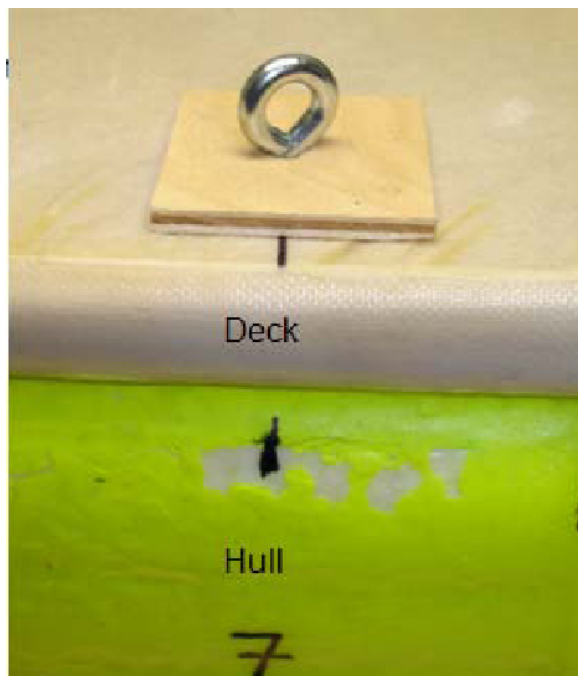
Figure 9-23. Deck and hull mounted together
