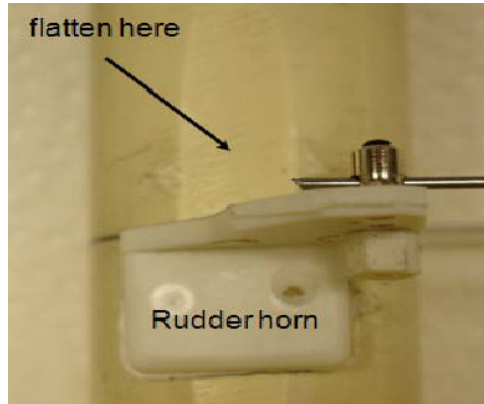
Figure 9-30. A rudder horn, glued to the tube
