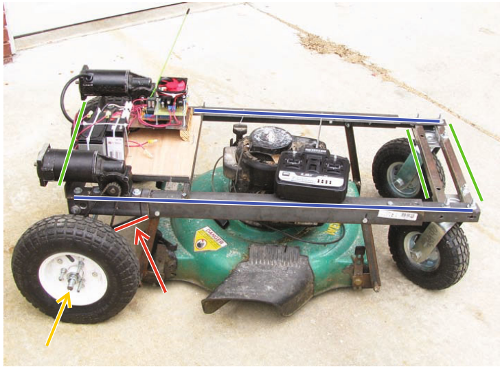
Figure 10-7. The axle and frame support bar
