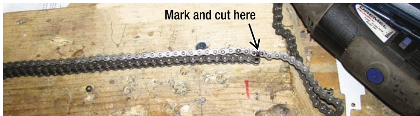
Figure 12-17. Measuring and cutting the chains
