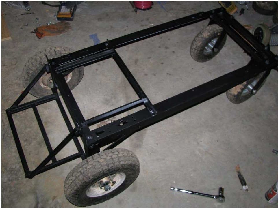
Figure 10-10. The completed frame
