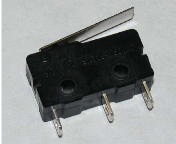
Figure 2-21. A typical tactile bump-switch with lever
