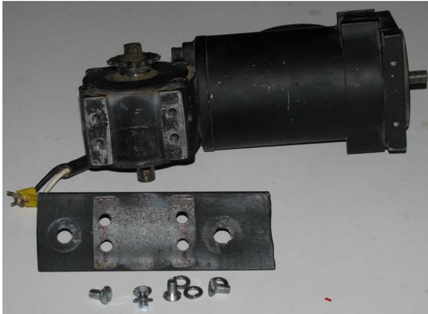
Figure 10-13. The motor mounting plate with 1/4-inch bolts
