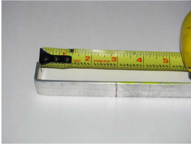
Figure 5-15. The side sensor brackets were made from a piece of 3/4-inch wide aluminum flat bar.
