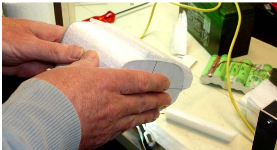
Figure 9-11. Fine cutting of one segment
