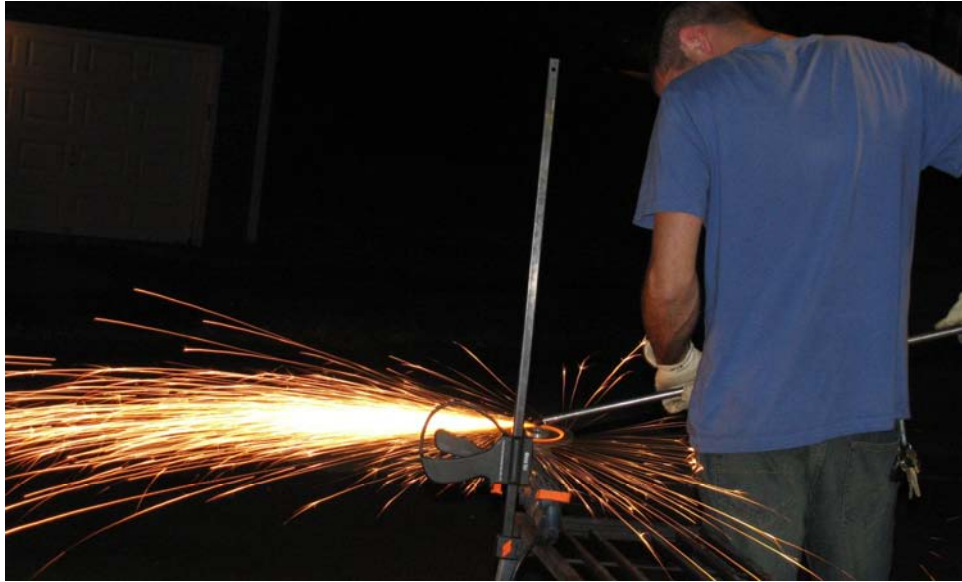
Figure 12-33. Grinding the spikes to make sharp points
