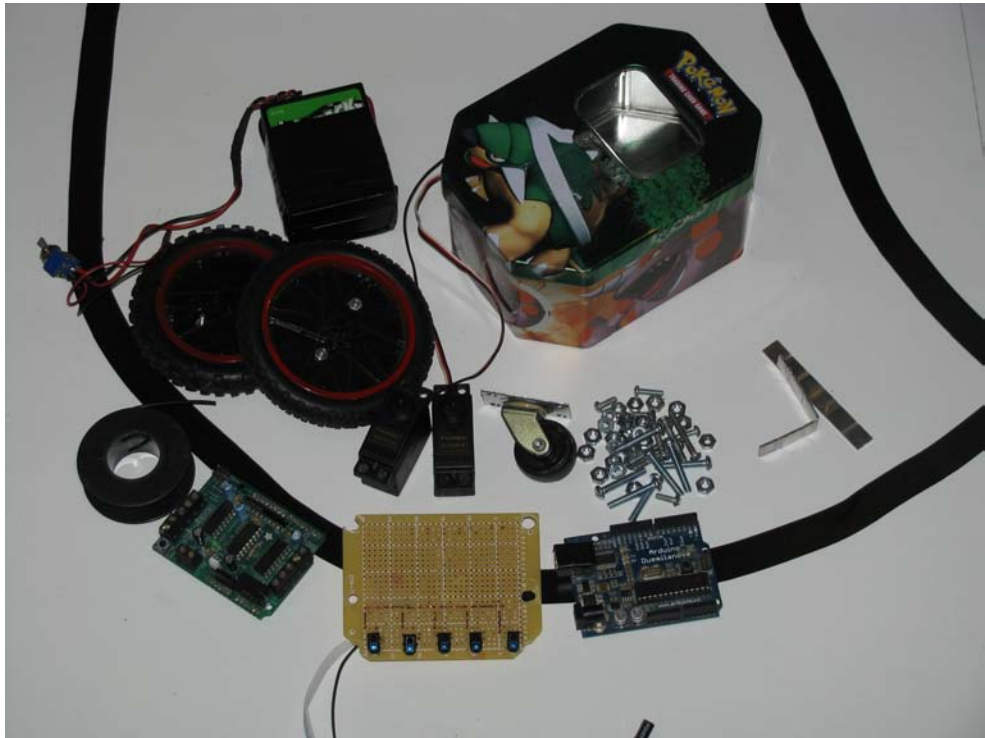
Figure 4-2. Here you can see the unassembled parts used to build Linus.
