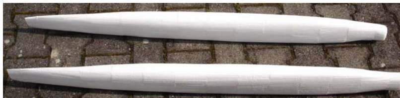
Figure 9-14. All segments glued together
