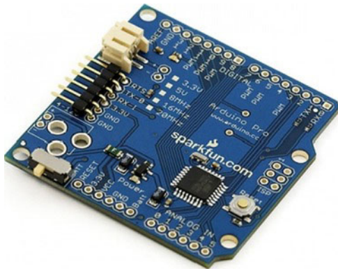
Figure 1-15. The SparkFun Arduino Pro is a stripped-down, minimalist Arduino circuit. It requires an external USB adapter to upload sketches. Photo by SparkFun. Used with permission.
