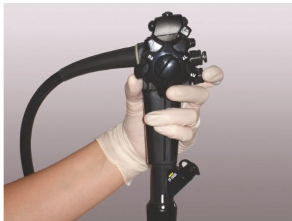
Fig. 6.1 Correct positioning of the left hand on the head of a colonoscope
