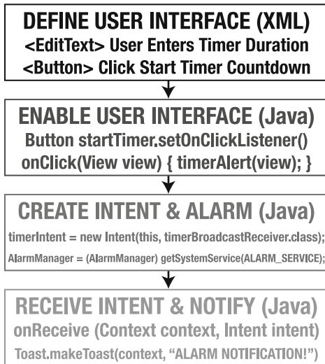
Figure 11–19. What we have to do in XML and Java to create the intent and alarm
