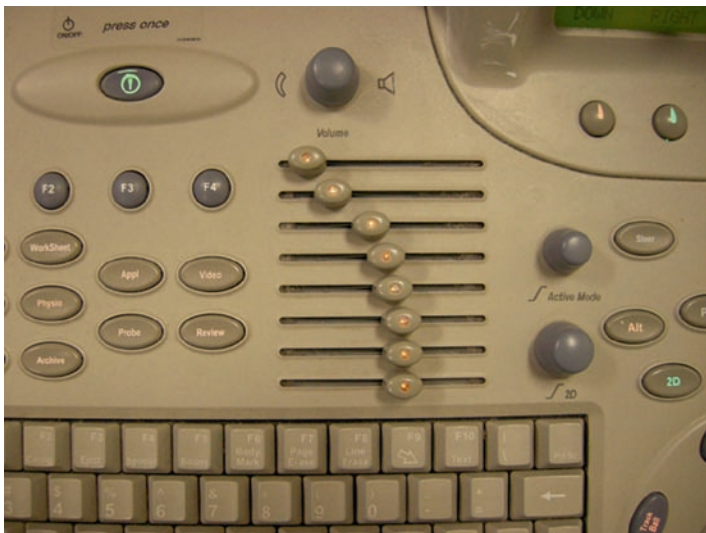
FIGURE 1.8. Time Gain Compensation slide potentiometer aligned in a curve (recommended starting position).
