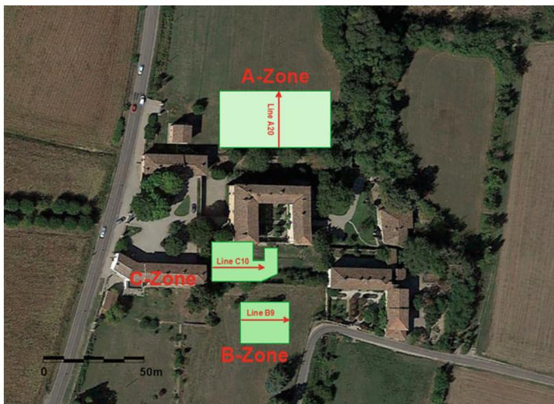
**Fig. 4.21** A sketched map of the Castle of Zena (C-shaped central light blue area) and the three ERT A, B, and C survey zones (grey areas). The red lines A20, B9, and C10 are the profiles selected to show examples of the nature of the input data in the form of 2D pseudosections
