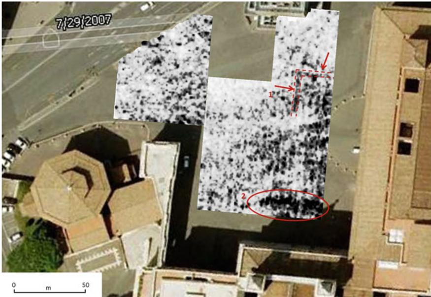
**Fig. 4.43** St. John Lateran square. Area A1 and B1, GPR 70 MHz, slices at the estimated depth of 6.00 m
