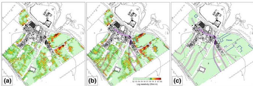
**Fig. 4.104** The electromagnetic induction survey: **a** map of electrical resistivity; **b** map of electrical resistivity with indication of anomalies; **c** map of anomalies
