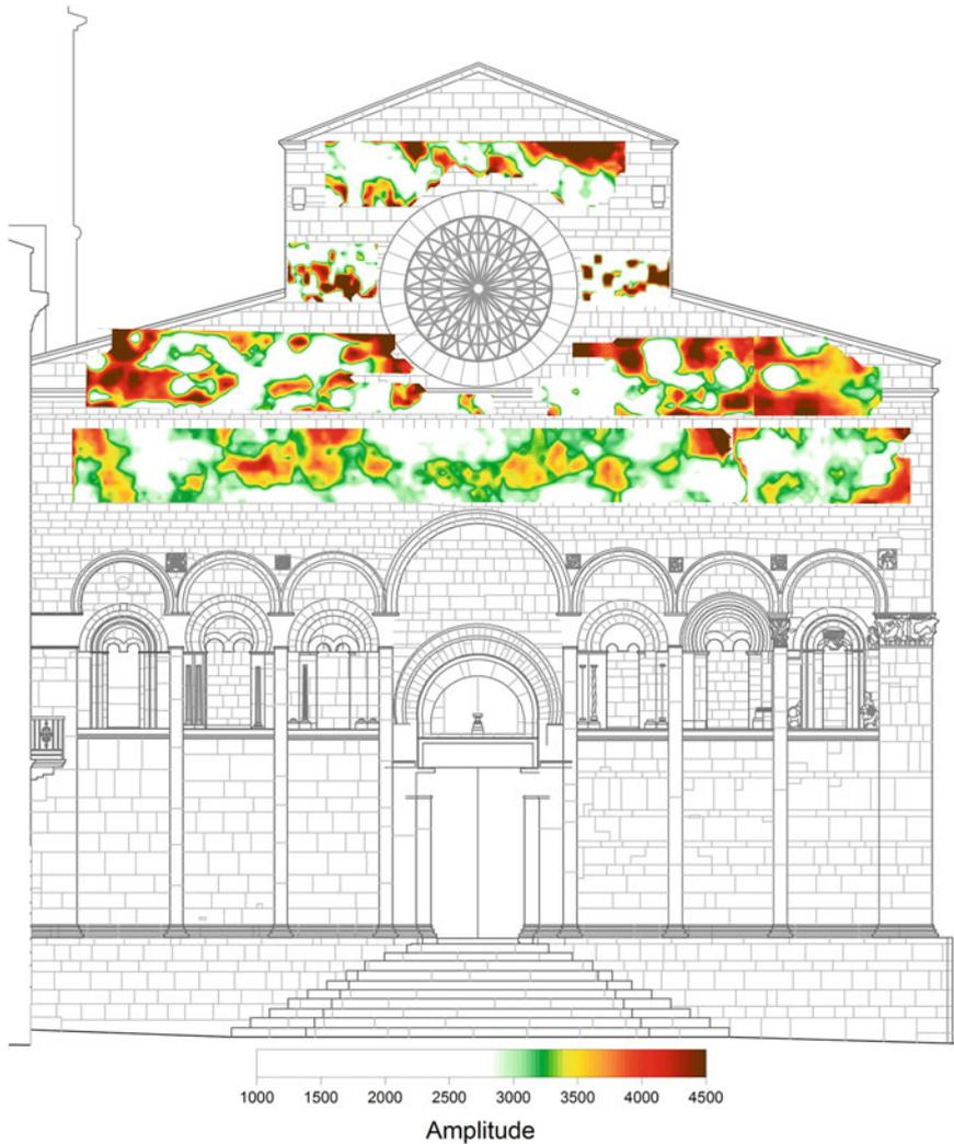
**Fig. 4.45** Slice in the time window from 5 to 10 ns (two way time)
