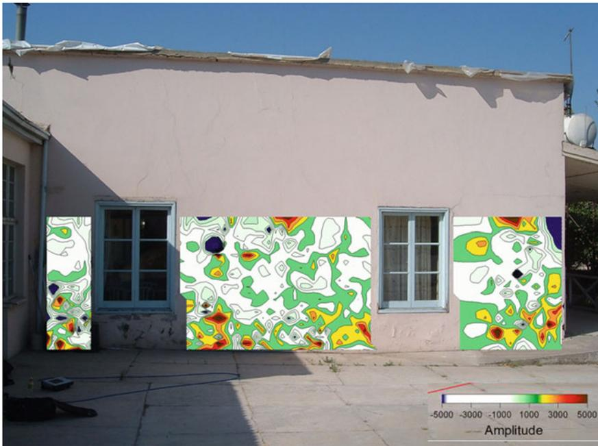
**Fig. 4.51** Vertical GPR slice
