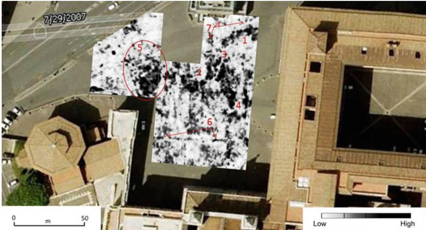
**Fig. 4.40** St. John Lateran square. Area A1 and B1, GPR 400 MHz, slices at the estimated depth of 0.88 m
