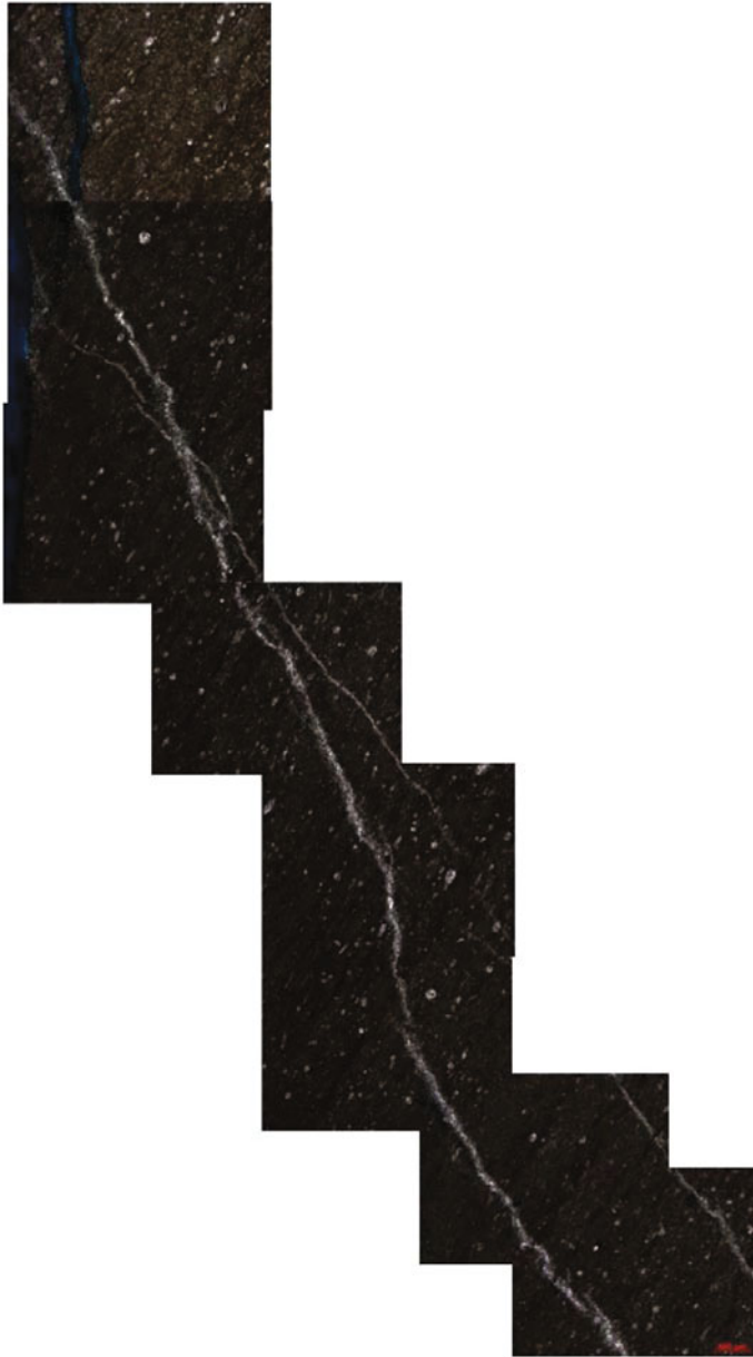
Fig. 6.12 Photomosaic. Micrit matrix with radiolarian, and cemented fractures. Taken with crossed Nicols (2.5X)
