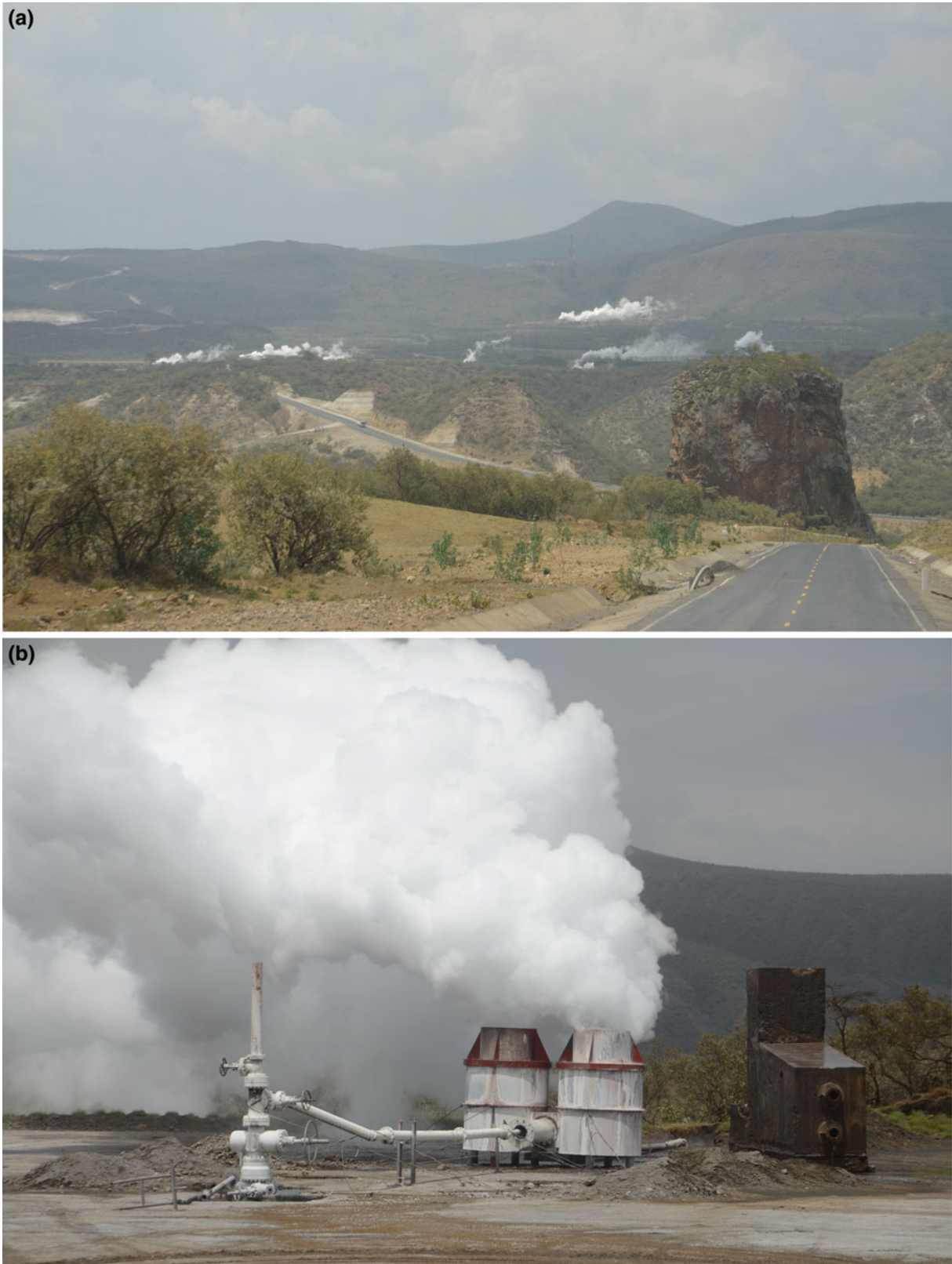
Plate 3.3 a The Olkaria geothermal field, Hell's Gate National Park is exploiting heat from a relatively shallow magma chamber; b Steam is vented from wellheads under excess pressure
