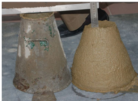
Fig. 2. Deformation graph for slump test of conditioned soil
