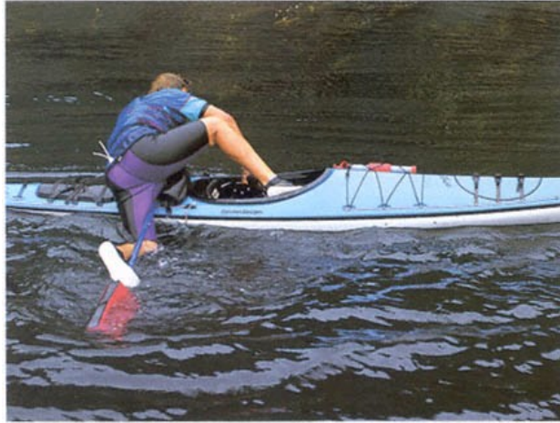
A paddle float acts as an outrigger to stabilize the boat for reentry.
