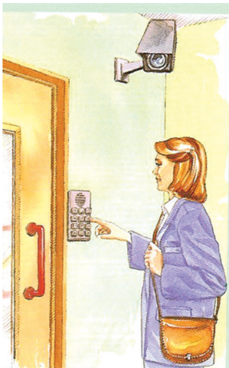
Figure 17.13 Security access and surveillance CCTV camera.
