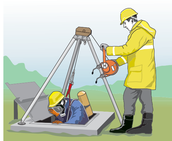
Figure 6.8 Entering a confined space.
