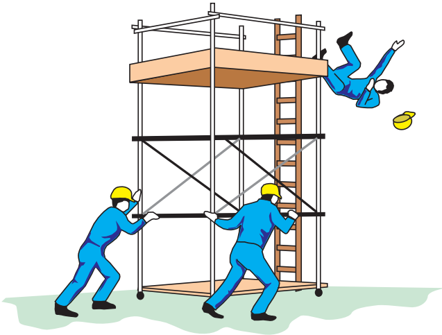
Figure 11.3 Falling from a height – tower scaffold.
