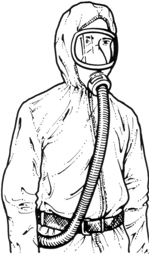
Figure 6.3 Respiratory protection and disposable overalls are needed when working in higher levels of asbestos dust.
