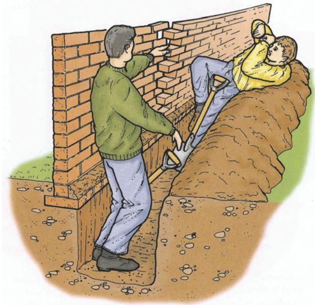
Figure 9.2 Undermining of boundary wall.
