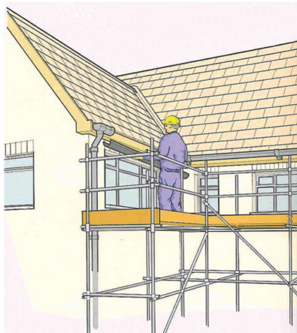
Figure 8.9 (a) Typical independent tied scaffold; (b) fixed scaffold left in place to fit the gutters.
