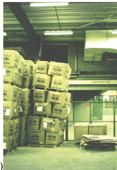
Figure 11.6 (a) Internal roadway with appropriate markings; (b) unsafe stacks of heavy boxes.
