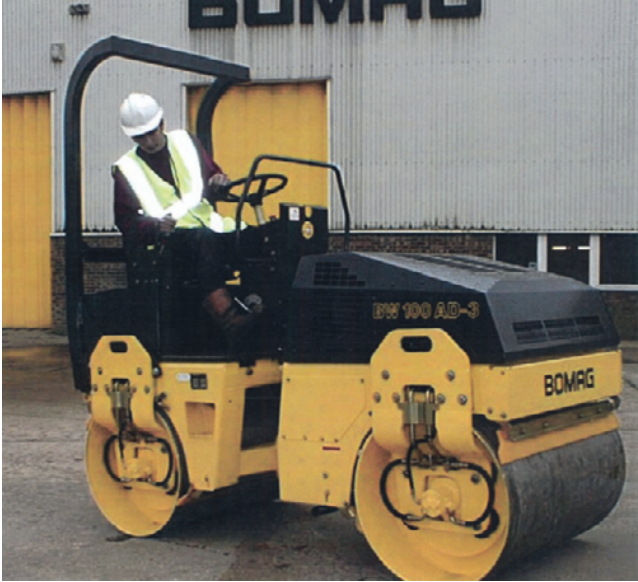
Figure 12.26 Ground consolidation vibrating roller.
