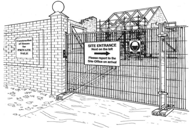
Figure 7.2 Secure site access gate.
