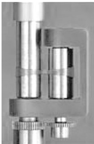
Fig. 6.19 Photo of extensional viscosity fixture (EVF) made by TA instruments. Courtesy of instruments courtesy of Catherine Jackson [80]
