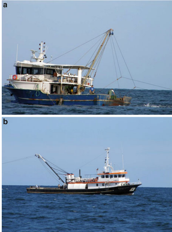
Fig. 23.2 Vessel used for beam-trawl R. venosa harvesting: length of 15 m (a) and 26 m (b) (original)
