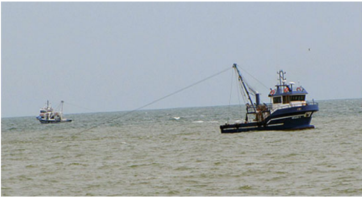
Fig. 23.5 Vessels over 12 m fishing with beam trawl
