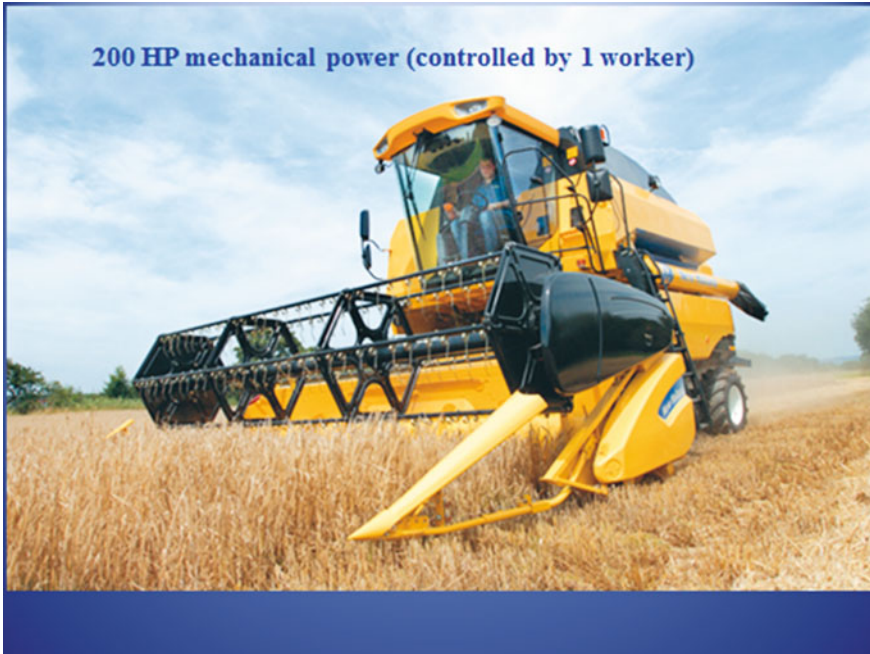
Fig. 9.3 200 horsepower fossil-fueled harvester, controlled by one person and not requiring fuel in the off-season. Other workers are required to make and repair the machine, and to provide the diesel fuel. Photo courtesy of Mario Giampietro
