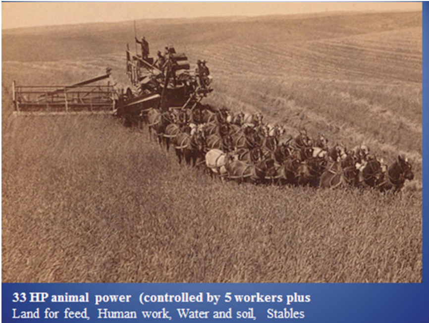
Fig. 9.2 33 Horsepower harvester. Controlled by 5 workers. In addition other workers were needed to till the land for horse food, water and feed the horses, muck the stables, etc. Photo courtesy of Mario Giampietro
