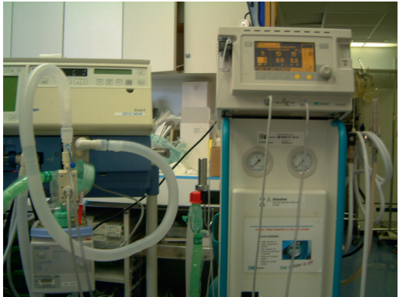
FIGURE 13.6. Photograph of the INOvent nitric oxide delivery system connected to a mechanical ventilator.
