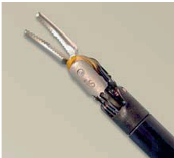
Fig. 8. The 8 mm PK ™ dissecting forceps (Intuitive Surgical Inc.) use electrothermal bipolar vessel sealing, an alternative bipolar energy form, which couples high current and low voltage.
