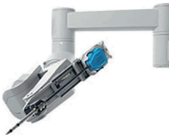
Fig. 5. The arms are equipped with two flexible joints, the proximal of which moves in the up/down, sideways, and rotational axis.
