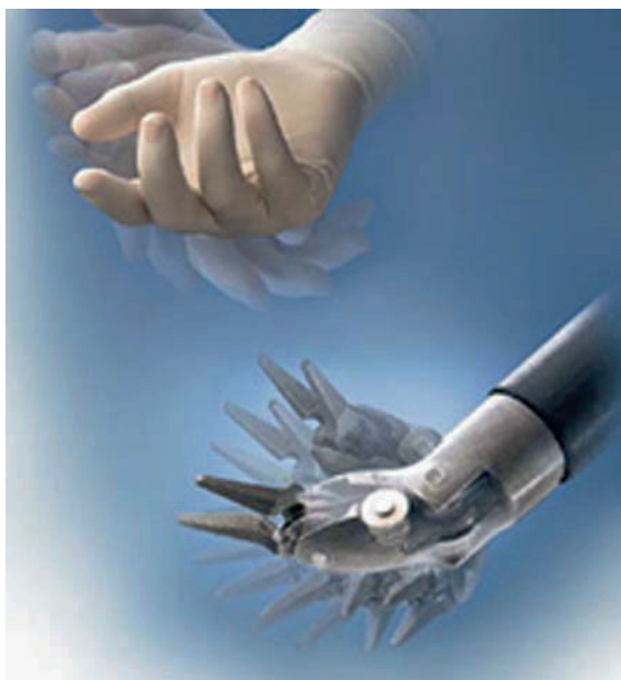
Fig. 1. EndoWrist ® instruments have a total of six degrees of freedom plus grip, mimicking the up and down and side-to-side flexibility of human wrist.
