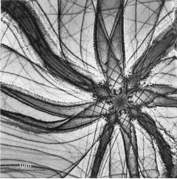
Fig. 9.3. Bend contours in a NIMONIC75 thin foil, forming a [100] zone-axis pattern (courtesy of P. Tambuyser).
