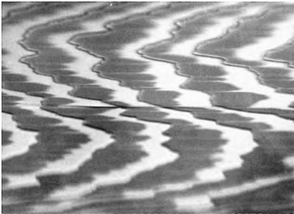
Fig. 9.42. Reflection electron microscope (REM) image of the (111) face of an Si crystal obtained with the (444) diffracted beam and showing the nucleation and growth of 7\times 7 structures (dark regions) at surface steps when the specimen is cooled from the transition temperature at 830^\circ\text{C} , where it shows the 1\times 1 structure (bright regions) (courtesy of H. Yagi).
