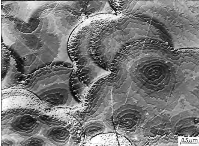
Fig. 9.40. Bright-field image of a 3.4 monolayer Au(111) film with a direction of incidence near \langle 315 \rangle . In addition to the contrast from different thicknesses due to the short extinction length, the steps are imaged by Fresnel-like black–white fringes due to phase contrast (courtesy of M. Klaua and H. Bethge).
