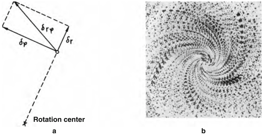
Fig. 2.17. (a) Chromatic error streak and (b) demonstration by superimposed focal series of polystyrene spheres.
